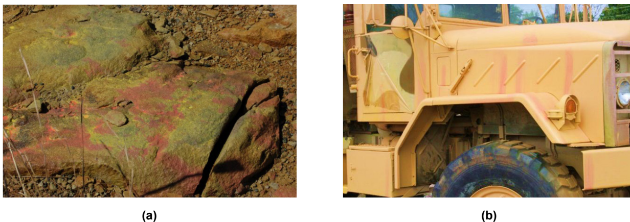
Figure 4-1: Disclosure Spray Indicating Contamination on Terrain (a) and a Vehicle (b) by Turning Red.
