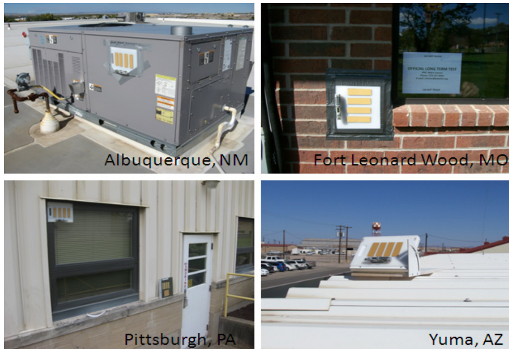
Figure 4-10: Coating Samples Were Exposed in Four Locales for a Period Up to 6 Weeks.
