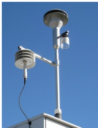
Figure 2-16: Example of Existing Sensor for Detection of Noxious Gases In or Near the Port of Rotterdam.
