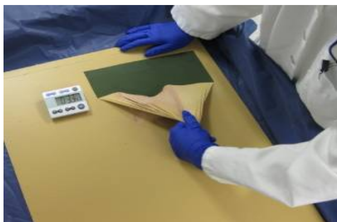
Figure 4-6: Strippable Coat Can Be Applied to a CARC-Coated Surface and Easily Scored, Peeled and Removed.
