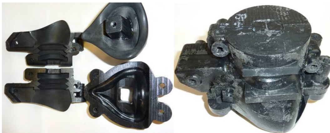
Figure 3-39: The Mold Tool Used to Create the Silicone Oro-Nasal Mask Shown in Figure 3-40(a).
