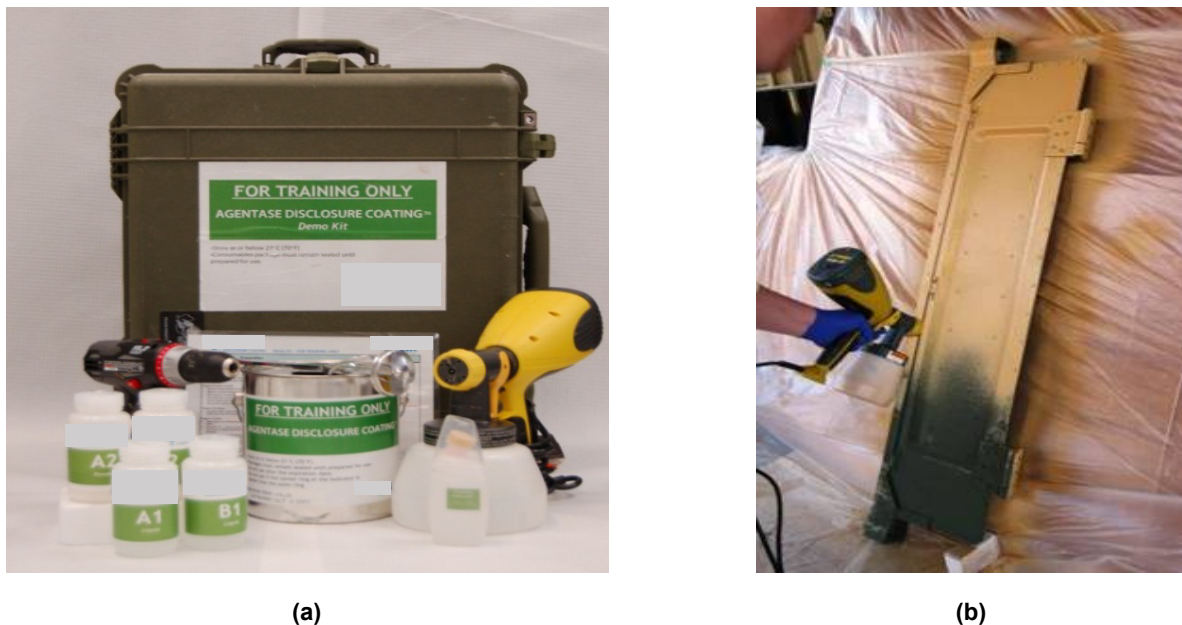
Figure 4-7: The Disclosure Coating Prototype Consumable (a) Contains Dried Powders (the user simply adds water to dissolve and stirs the additives into the coating) – Once Mixed, the Coating is Loaded into a Standard HVLP Sprayer (b) and Applied.
